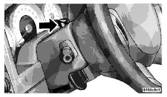
This is an emergency warning system and should not be used when the vehicle is in motion. Use it when your vehicle is disabled and is creating a safety hazard for other motorists.
